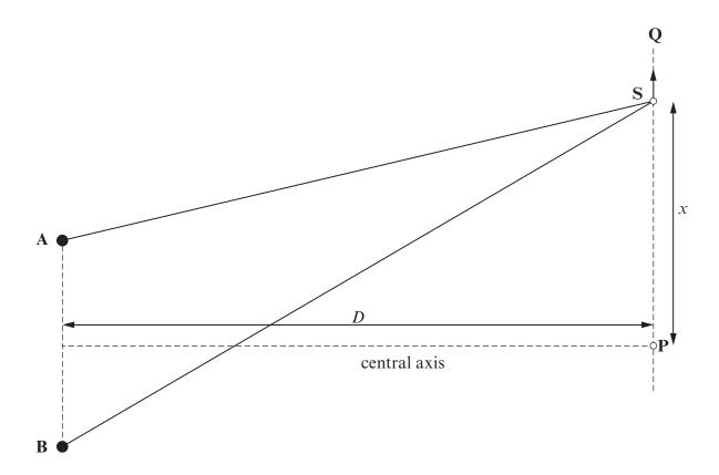
As a microwave sensor, S, is moved from P towards Q, the intensity is found to vary, with the first three maxima when x = 0, when x = 10.0 cm and when x = 22.0 cm.
